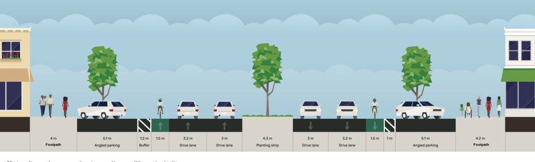
**Note:** dimensions vary due to on-site conditions, including width of linemarked buffer zone varies, minimum shown
